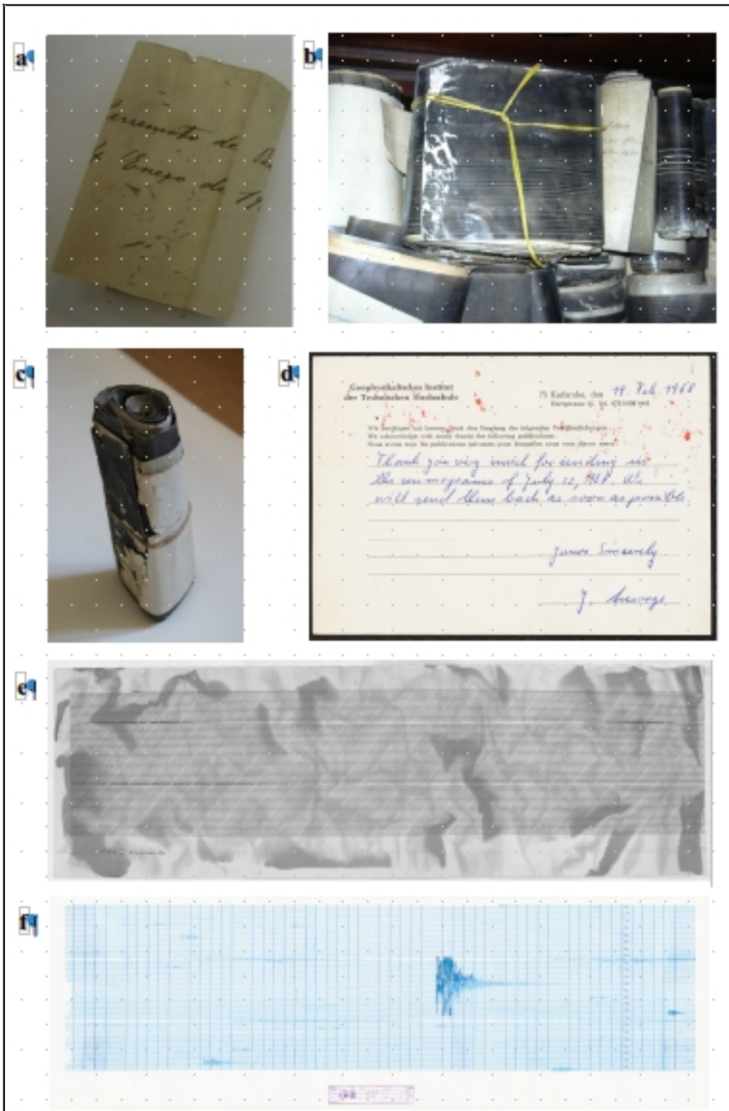
Figure 8. Some more examples of the diversity of problems about conservation risks: 8a) surface dirt; 8b) mechanical degradation due to improper storage; 8c) inadequate acidifying paper in direct contact; 8d) ink spots; 8e) degradation of chemical components; 8f) ink attenuation because of excessive exposition to sunlight. Source: Observatori Fabra.
